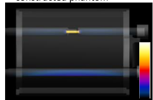
Figure 2: Sagittal view of simulated SAR distribution for the phantom in position 1. Very localized SAR is realized inside the narrowed tube compared to the straight tube
